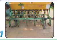
Measure the width of the seed drill by placing one end of measuring tape at middle of first tyne and other at middle of last tyne and note the width in a note pad. Add 20cm (row to row spacing) to the width of seed drill to arrive at effective width of seed drill (or multiply no. of tynes by row spacing to arrive at effctive width of seed drill).
