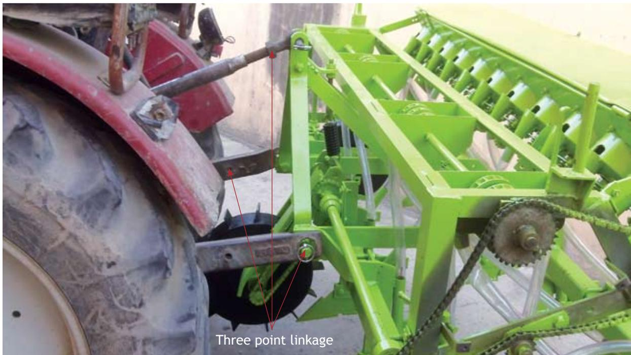
**Figure 26.** Hitching of machine through three-point linkage
