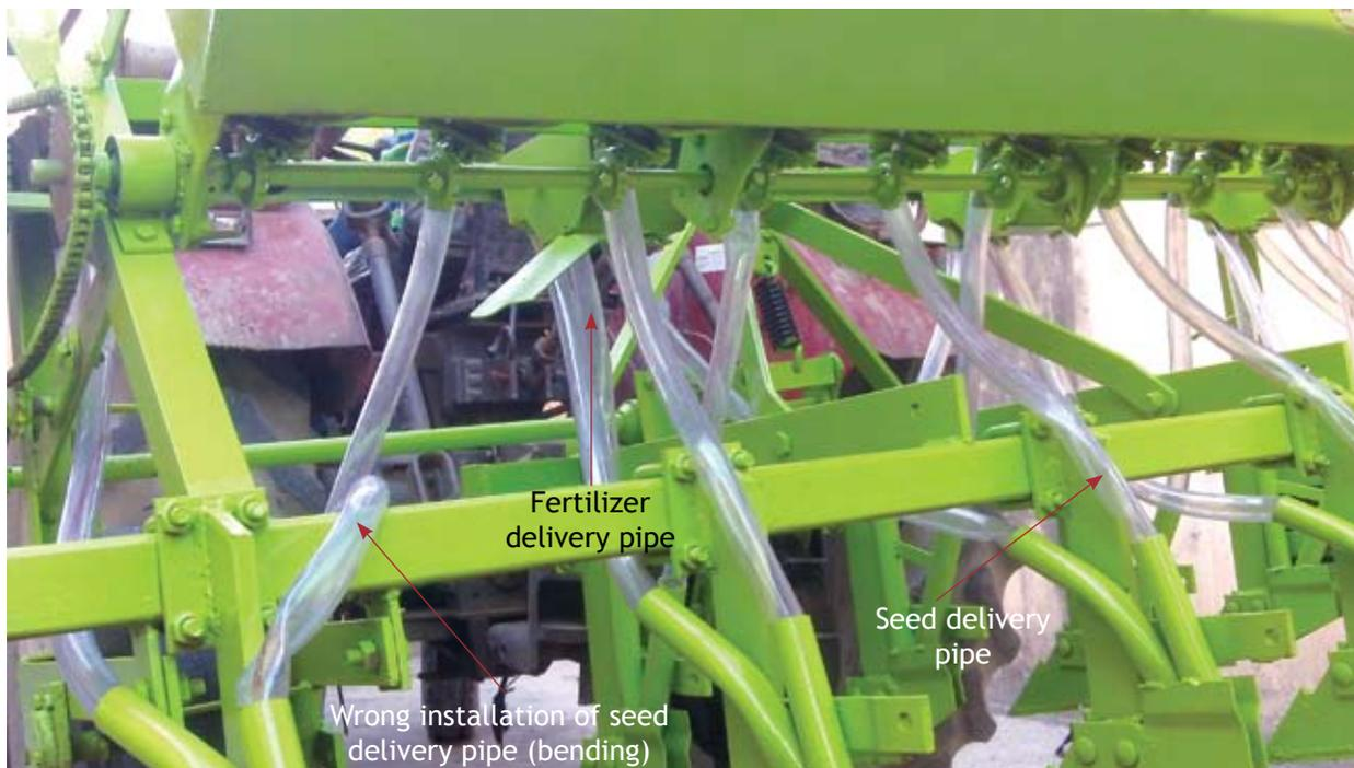
**Figure 22.** Seed and fertilizer delivery pipes
