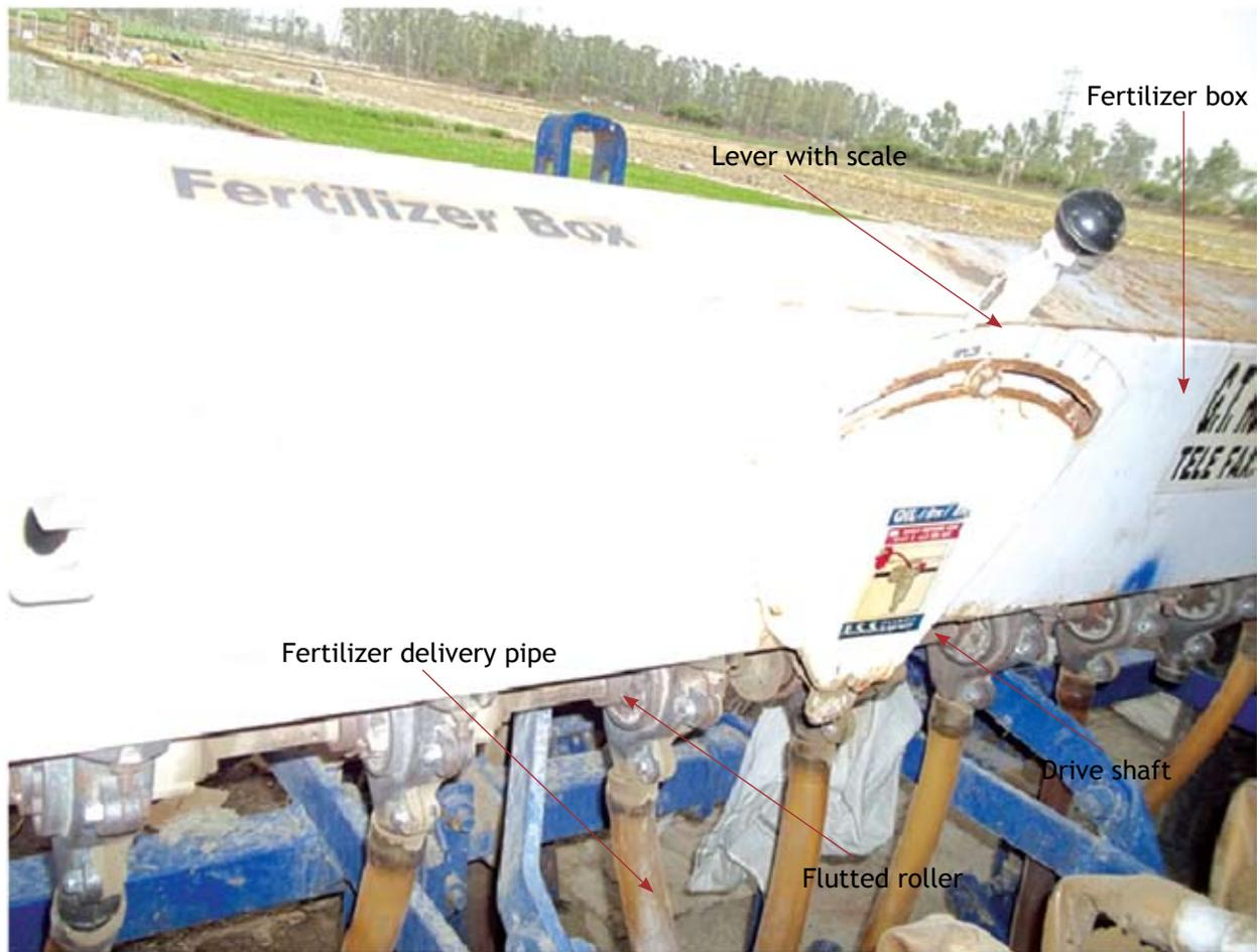
**Figure 11. Fertilizer metering system**
