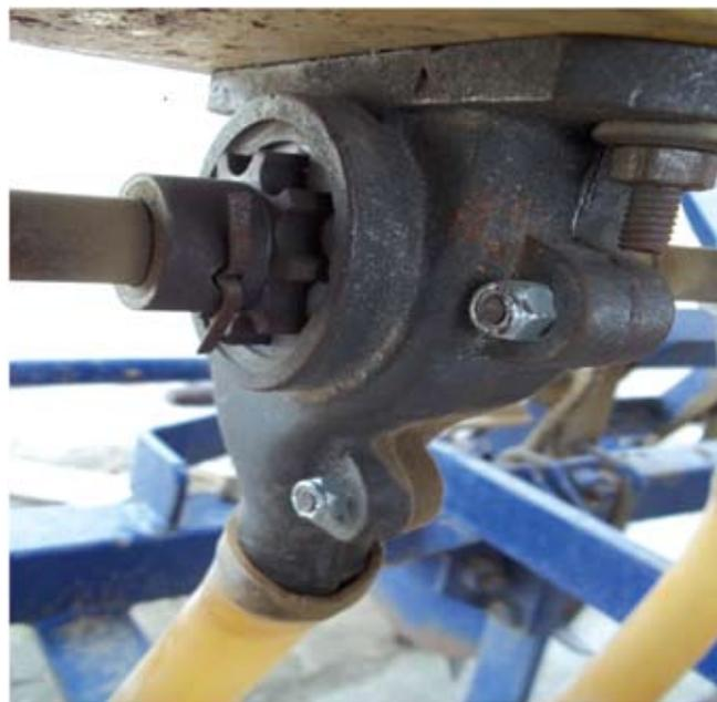
**Figure 12. Fluted roller with shaft**
