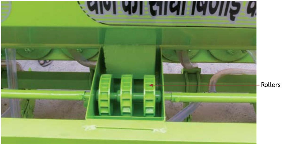
*Figure 17. Cup/cell type roller*
