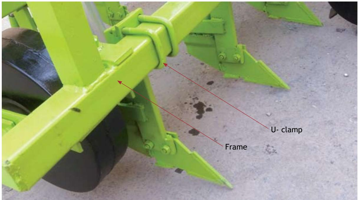
**Figure 2. Components of Frame and its adjustment**
