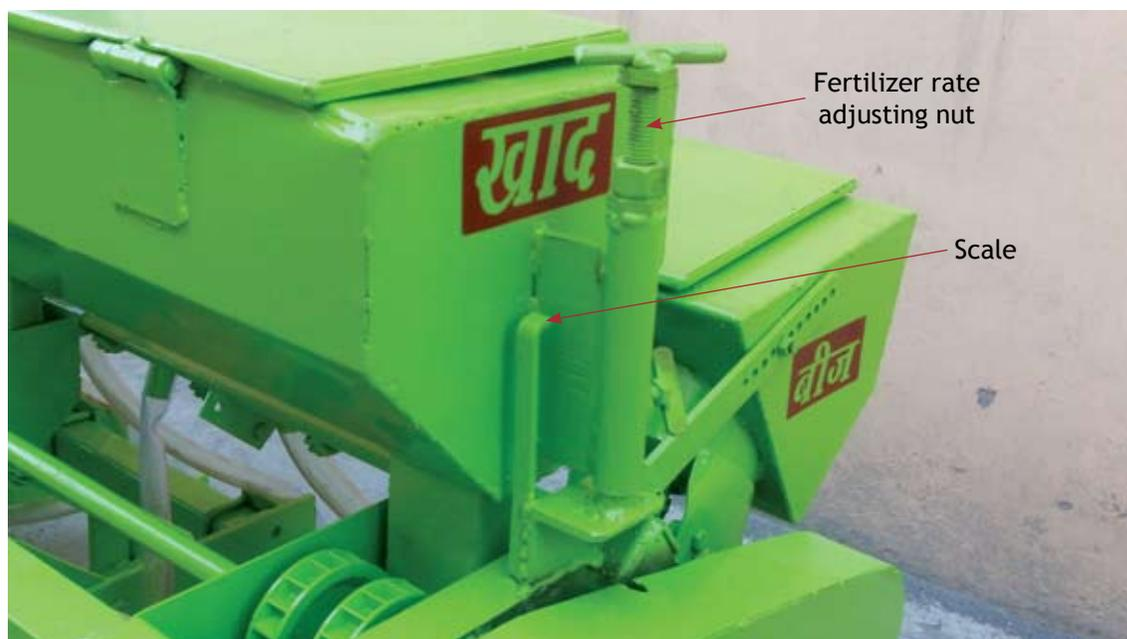
**Figure 16. Fertilizer rate adjustment**
