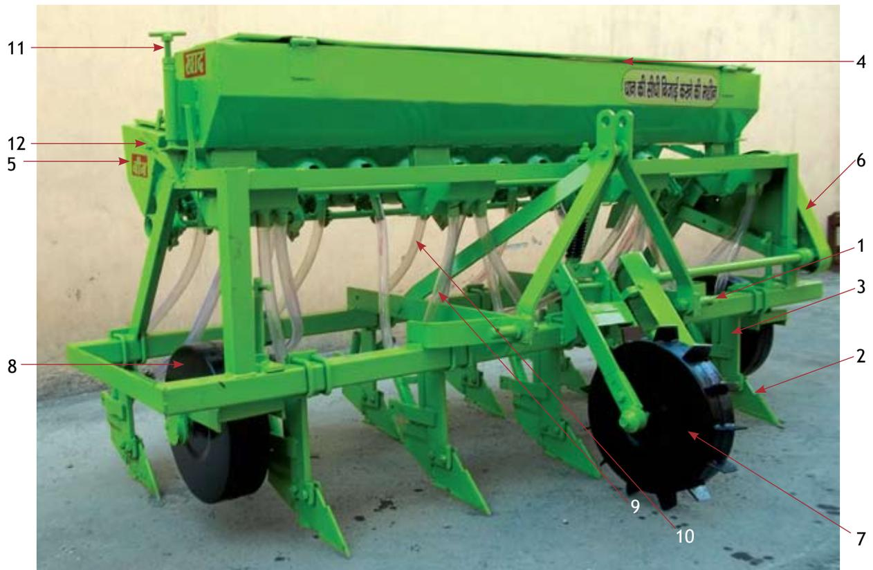
1. Frame, 2. Furrow openers, 3. Tynes, 4. Fertilizer box, 5. Seed box, 6. Chain and gear drives, 7. Drive wheel, 8. Depth control wheel, 9. Fertilizer delivery pipe, 10. Seed pipe, 11. Fertilizer rate adjusting nut, 12. Seed rate adjusting strip
