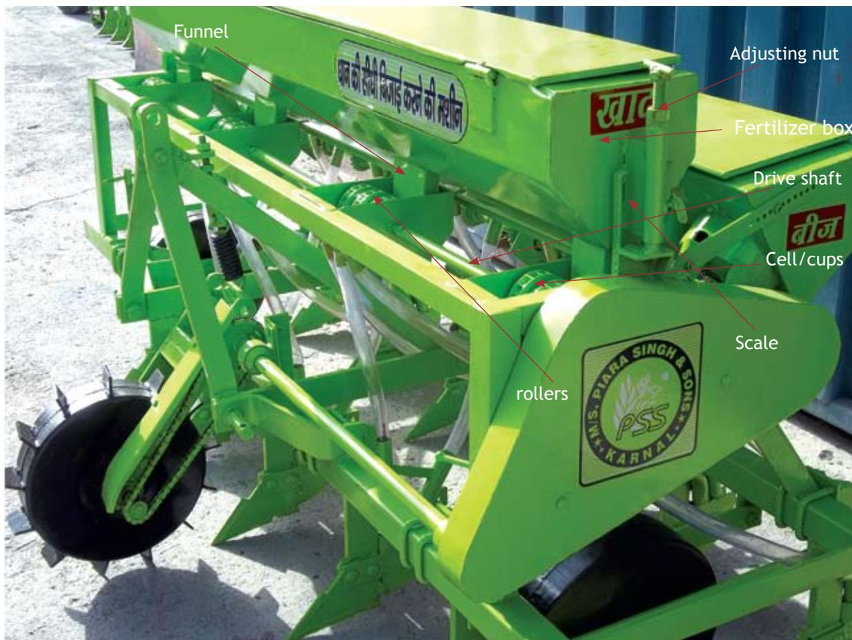
**Figure 15. Fertilizer metering components**
