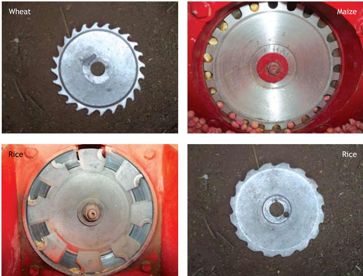
*Figure 10. Types of inclined plates used in multi-crop planter*
