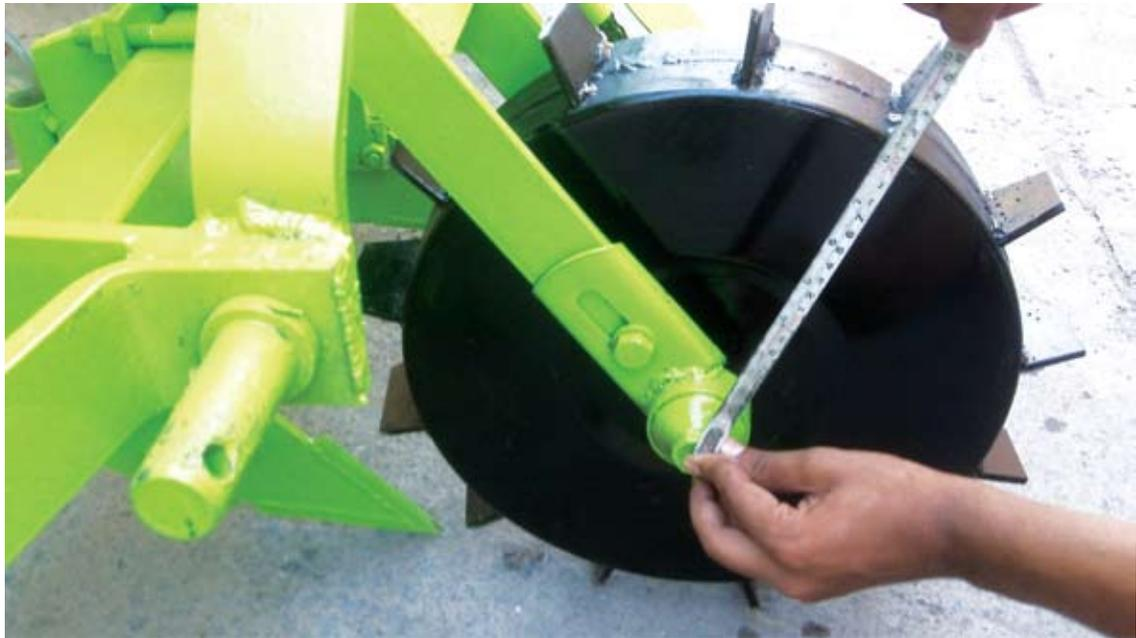
*Figure 24. Diameter of drive Wheel*
