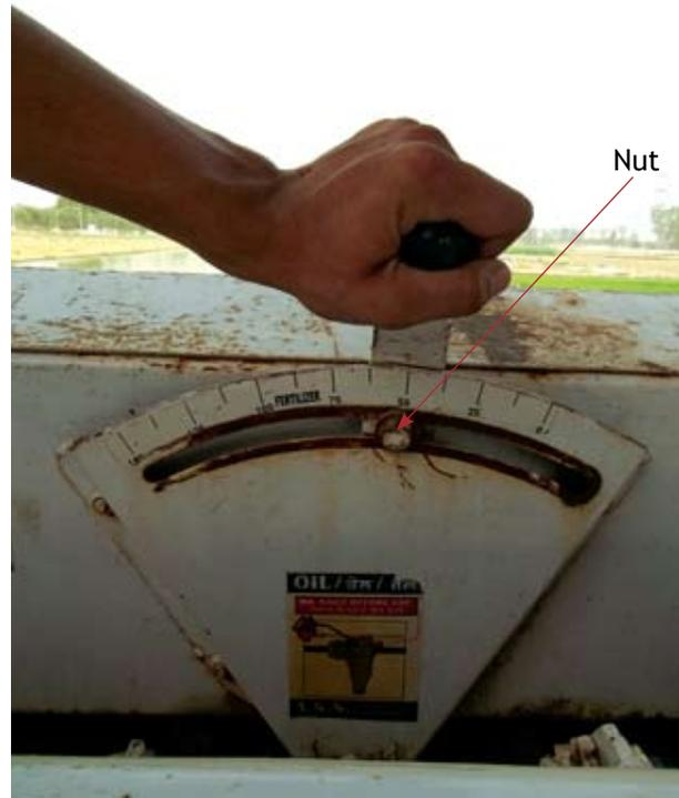
**Figure 14.** Fertilizer rate adjustment lever with scale and nut
